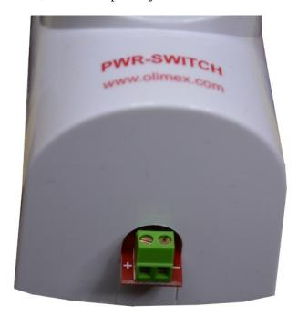
If you want to drive PWR-SWITCH with Arduino you should connect the green termianl with "–" to GND and the terminal with "+" to Arduino D0 pin. Here is the code to switch it on and off:
