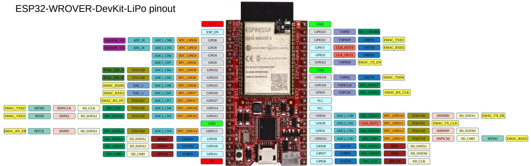
GPIOs which are not available: GPIO6, GPIO7, GPIO8, GPIO9, GPIO10, GPIO11 internal SPI Flash
