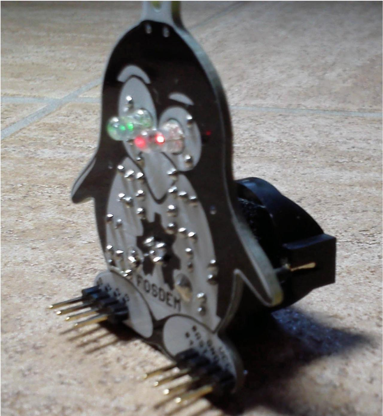
I bought a FOSDEM-85-penguin from the Olimex web shop. After some days it arrived in Germany. I soldered it without any problem. It looks nice so I decided to give it a place at my desk as a thermometer. I use the ATTiny85 internal chip sensor for measuring the temperature.
